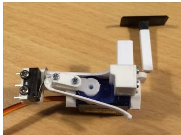
Figure 1: Hugo Fitzjohn's uncoupler mount
