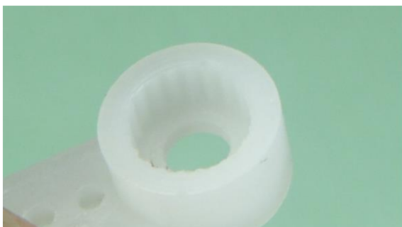
Figure 2: Splines inside servo horn
