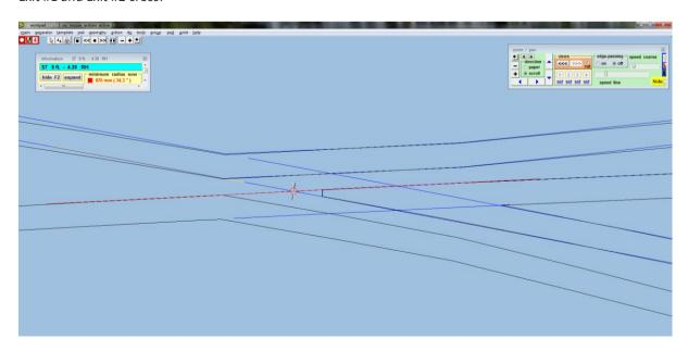
Set geometry  $\rightarrow$  peg positions  $\rightarrow$  peg on FP (CTRL-4). Set action  $\rightarrow$  F5 V-crossing angles  $\rightarrow$  any angle and action  $\rightarrow$  F5 sizing options  $\rightarrow$  length locked. Use action  $\rightarrow$  mouse actions: real  $\rightarrow$  adjust turnout size only (F5) so that the vee of the turnout matches that of the crossing formed of Exit #1 and Exit #2:
