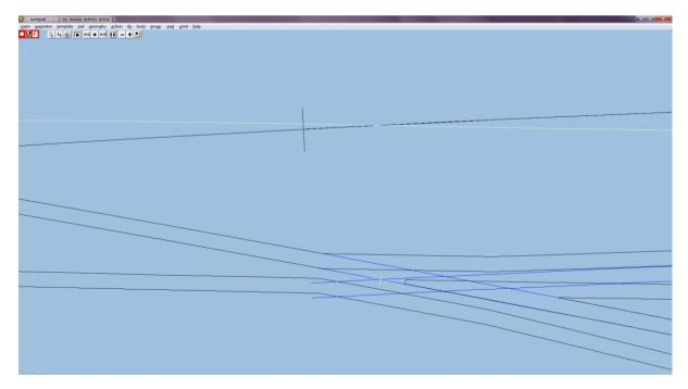
Set geometry  $\rightarrow$  peg positions  $\rightarrow$  peg on FP (CTRL-4). Set action  $\rightarrow$  F5 V-crossing angles  $\rightarrow$  any angle and action  $\rightarrow$  F5 sizing options  $\rightarrow$  length locked. Use action  $\rightarrow$  mouse actions: real  $\rightarrow$  adjust turnout size only (F5) so that the vee of the turnout matches that of the crossing formed of Exit #1 and Exit #2. Finally, unset geometry  $\rightarrow$  track centre-lines:
