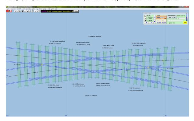
To get the Vee rail joints on the turnout roads it's necessary to show timbering on the Turnout closure templates (real  $\rightarrow$  timbering  $\rightarrow$  equalized – constant), and then omit all of the sleepers by using the shove timbers tools (real  $\rightarrow$  shove timbers (CTRL-F10)), and click the omit all button.
