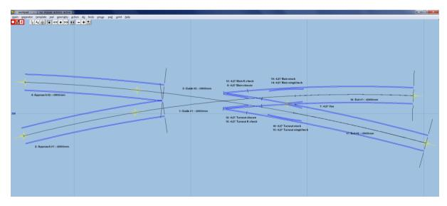
Note: the exit rails #1 and #2 might not line up directly with the appropriate stock rails at the vee. This can be accommodated during construction, or if it offends too much, duplicate the Exit #1 and Exit #2 and make these longer (into the diamond), and omit the appropriate rails.
