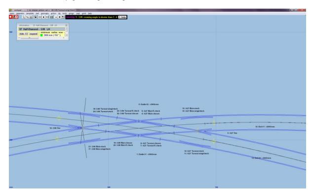
The following templates should have their timbering shown: 4.27 Main wing/check, 3.86 Main wing/check, 4.27 Main closure and 3.86 Main closure. The style should be equalized – constant with timbers centralised. Although you might want to double check with your chosen prototype company for exact timbering data.
