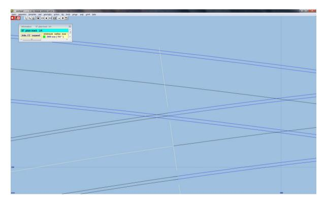
Select main  $\rightarrow$  store & background (CTRL-V). Left click on Guide 1 and select copy from control from the popup menu. Then select geometry  $\rightarrow$  peg positions  $\rightarrow$  peg on joint (Ctrl-1). Use action  $\rightarrow$  mouse actions: geometry  $\rightarrow$  adjust plain-track length (F4), and adjust the length of plain track until it is on the inside of the second vee:
