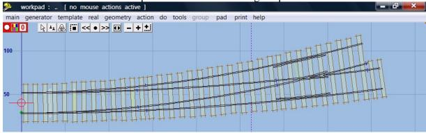
1. This "how to" is done with PUG .091c in S gauge. Start with B8 LH turnout, radius 10 chains. Change the main road curving to 3000 mm radius, timbers square on to main road.
