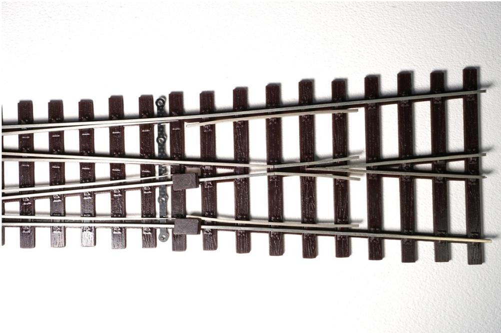
Soldering is done while the Switch Blades sits flush against the Stock Rails as this ensures best alignment. If you notice a gap between Switch Blades and Stock Rails, this can be taken up by squeezing them together at the top of the rail head with a small pair of tweezers, whilst soldering.
