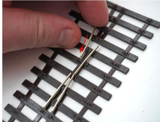
**IMPORTANT!** The join between the Wing Rails and the Closure Rails **MUST** be located exactly at the 'Knuckle' position. This position will be different for each kit, so **you MUST refer to your kits downloadable template which will show the exact position of the knuckle**. There is also a small indentation on the plastic base indicating the precise position of the 'Knuckle' join. Repeat for the opposite side of the Slip.
