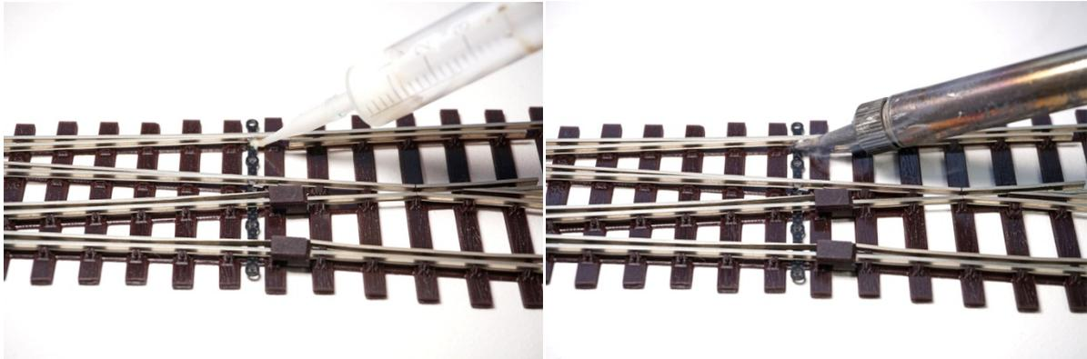
**NOTE: Please only use a small amount of solder, otherwise there is a risk of solder flowing under the Switch Blade and bonding the Switch Blade to the Stock Rail.**
