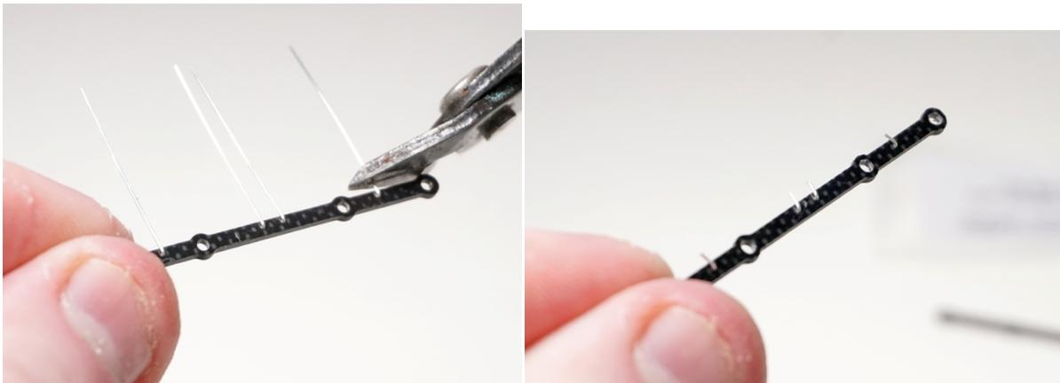
The pins can then be cut short leaving about 2 – 3mm of length as shown above.
