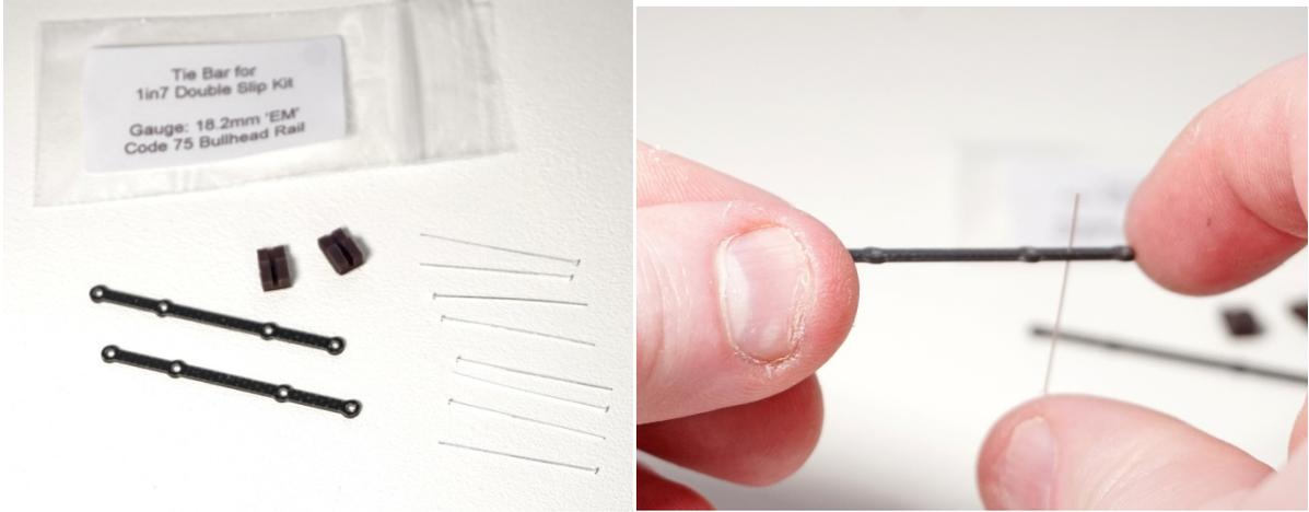
For each Tie Bar, 4 metal pins are inserted through the pre drilled 0.4mm holes in the tie base.
